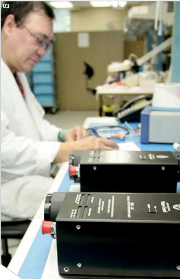
03. IWG A4 water treatment units being inspected 04. Layout of an IWG circulating water system on a VIP airliner
